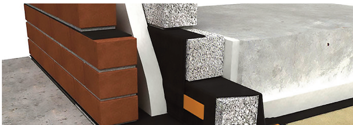
Fig. 11 | Anti-radon membrane, corner kit (credit: brooksonline.ie).
