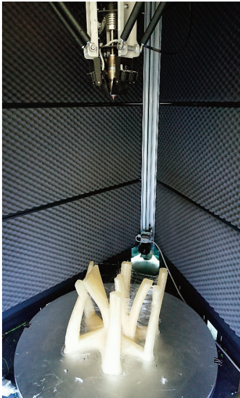
Figg. 9, 10 - D. Ficarra, Flux seat, Palermo 2018: phase of production and final product.
