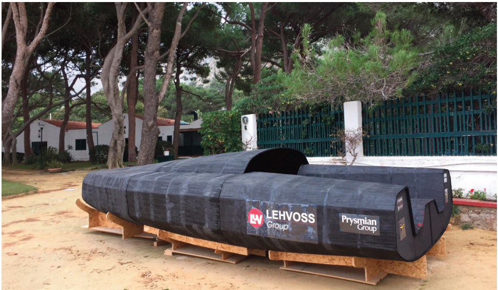
Fig. 16 - Mini 6.50 made entirely with additive manufacturing, Palermo 2018.
