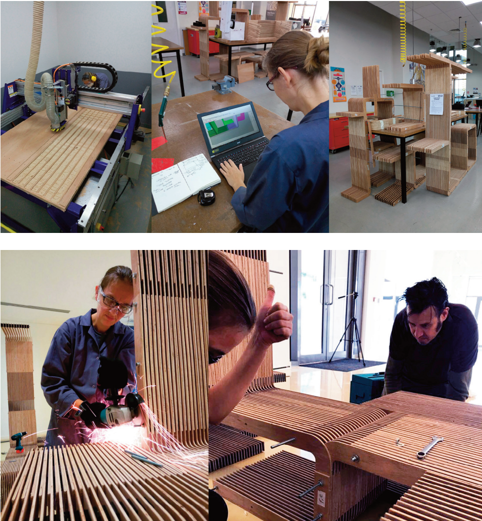
Figg. 4, 5 | Images of fabrication and assembling of the prototype (credits: Authors, 2018).
