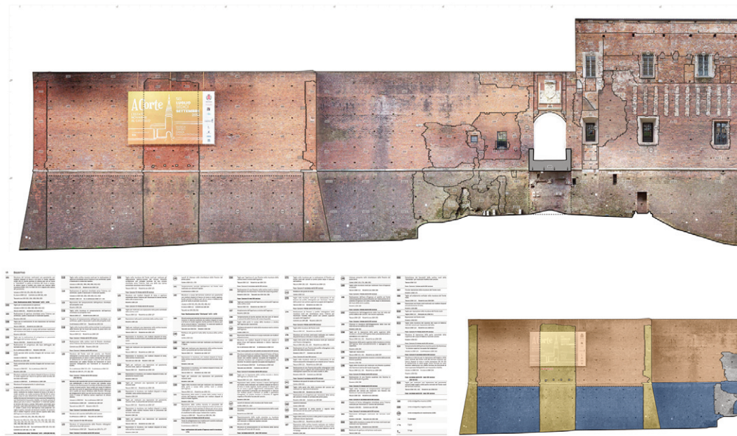
Figg. 17, 18 | Stratigraphic survey of the North facade of the Castle; Decay survey and maintenance project of South-North facade of the Castle (credits: Politecnico di Milano, DASTU and ABC Departments, F. Albani, M. Gambaro, 2018).
